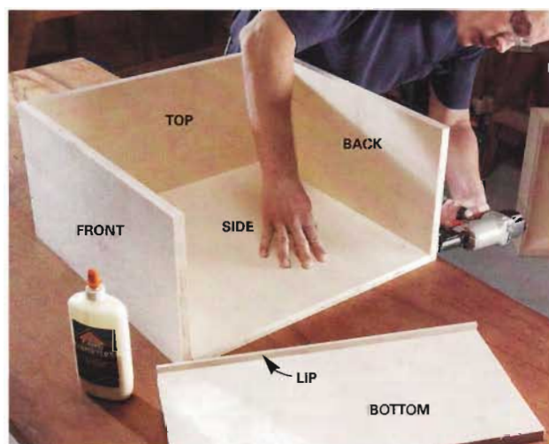
2 Assemble the boxes by gluing and nailing the front, top, back and bottom to the side panel and to each other. Nail the lip to the bottom shelf before assembling.
