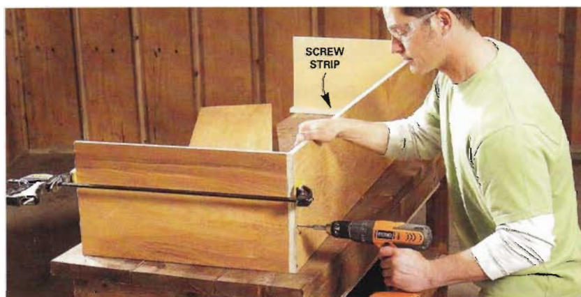
2 Clamp the frame parts together, including the screw strip. Drill pilot holes and drive screws.
