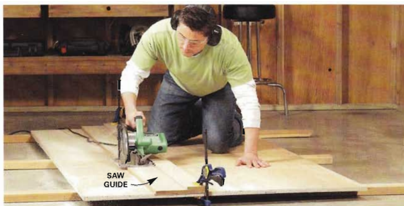
1 Get perfectly straight, accurate cuts with a circular saw using a homemade saw guide. Clamp the saw guide at your mark on the plywood.
