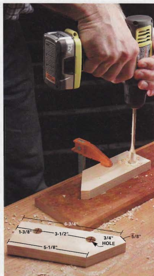
1 Clamp the 1x3 support to a piece of scrap wood as you drill the holes to prevent the wood from splintering.
