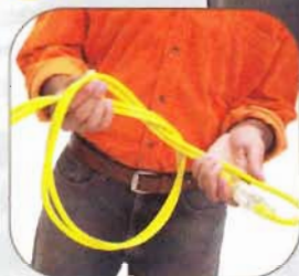
1 Fold the cord in half, then create a closed loop at one end.
